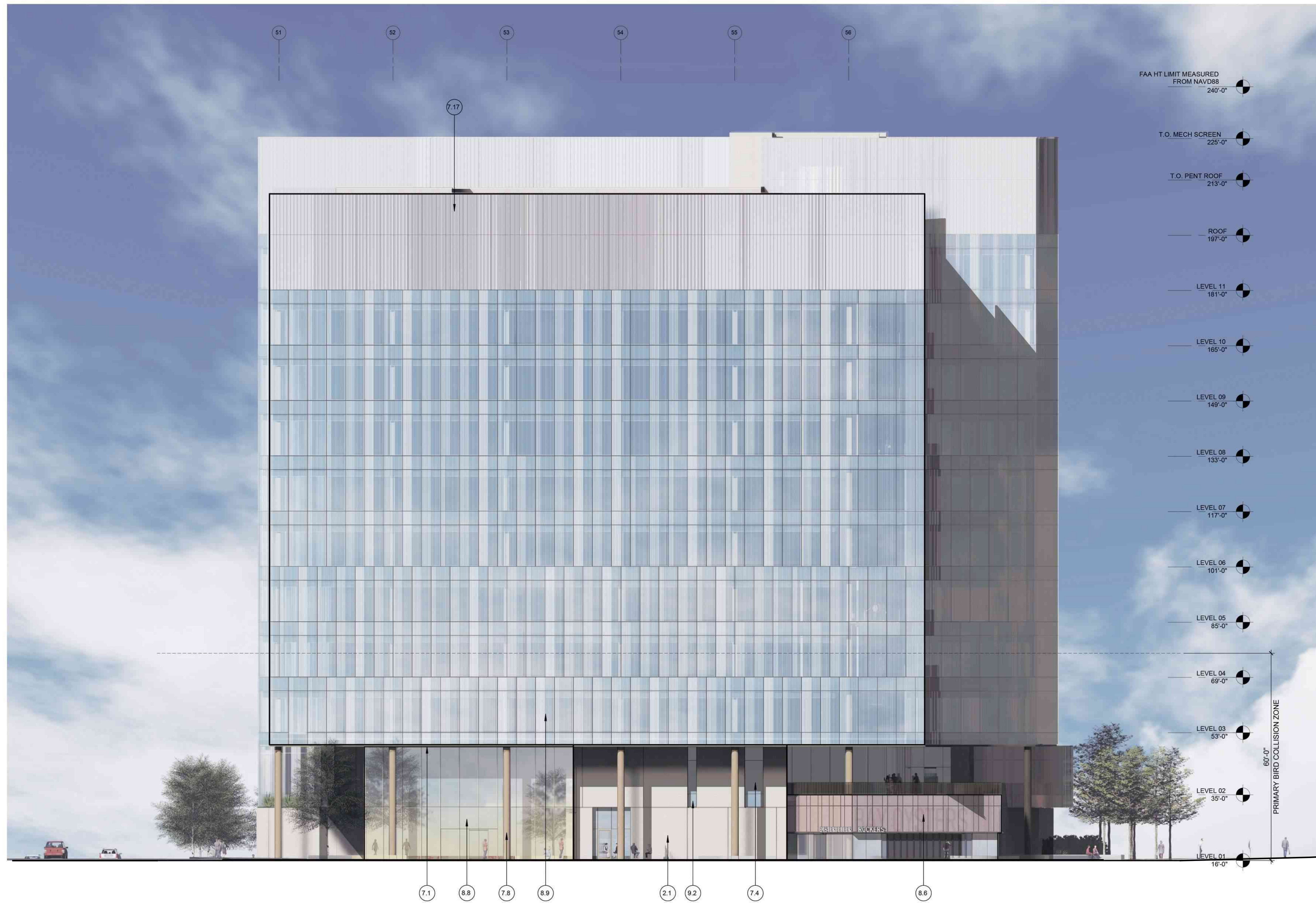
1 SOUTH BUILDING - AIRPORT BOULEVARD ELEVATION 1/16" = 1'-0"
